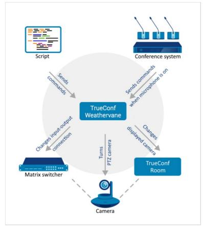
The following picture gives an example of how a meeting room equipped with PTZ cameras and TrueConf Room connected via TrueConf Weathervane may look like.
